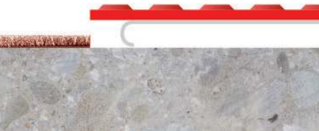
Image 5b – Peel and stick Adhesive: Recessed to floor finish on solid substrate.
